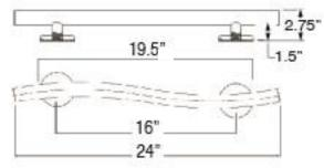
Easy to mount flange! 3 Set Screws on post allow pre-mounting to the wall before attaching the bar.
