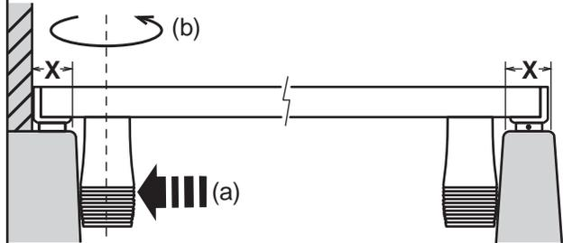
**BUMPER INSTALL.** If required, install the extra bumpers directly to the wood. Carefully drill a pilot hole for the (supplied) #6 pan head wood screws. Ensure the bumpers are aligned with factory-installed bumpers as shown in Bottom View.
